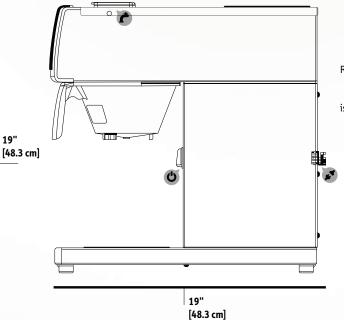
Recommended clearance for proper operation of Pourover Coffee Brewer is **30" [77.0 cm]** from top of the counter.
